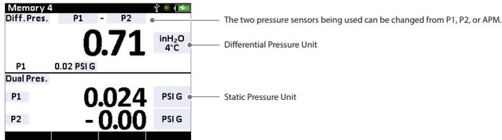
**Note:** The static pressure is also displayed on the bottom of the window. The unit for the static pressure does not have to be the same as the differential unit.
